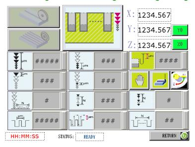
• Setting screen For Surface grinding & Criss-cross grinding
