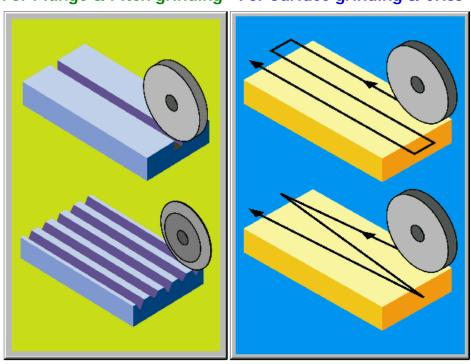
• Setting screen for Plunge & Pitch grinding
