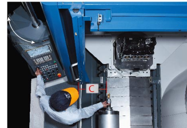
Access to spindle facilitates rapid tool changing.
