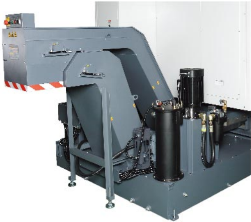
Coolant tank capacity HA-400II / HA-500II 550 L(80% full)
