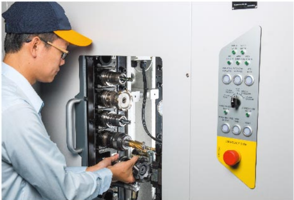
The tool magazine door design facilitates tool changing and checking. The operating distance and height is comfortable to operators.
