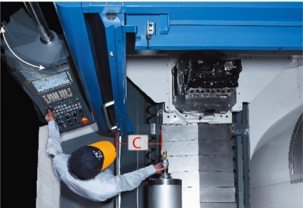
Access to spindle facilitates rapid tool changing.
