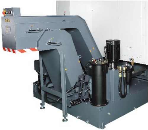
Coolant tank capacity HA-400II / HA-500II 550 L(80% full)
