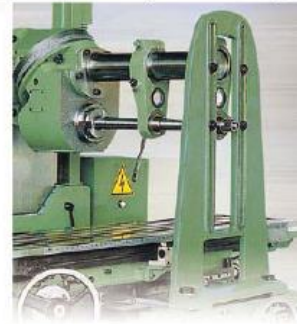
Horizontal milling arbor accessory
