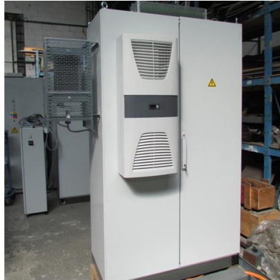
Electrical cabinet with cooling
