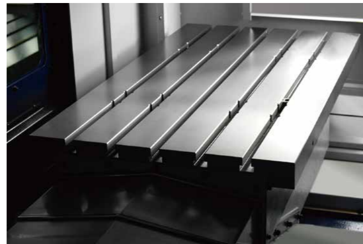
Fine ground table surface with excellent flatness.
