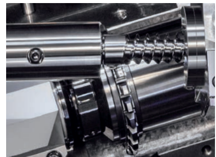
Worm-milling with milling cutter.
