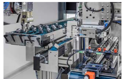
Direct loading/unloading to conveyor.
