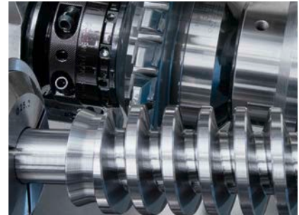
Worm manufacturing with regular HSS milling cutters.
