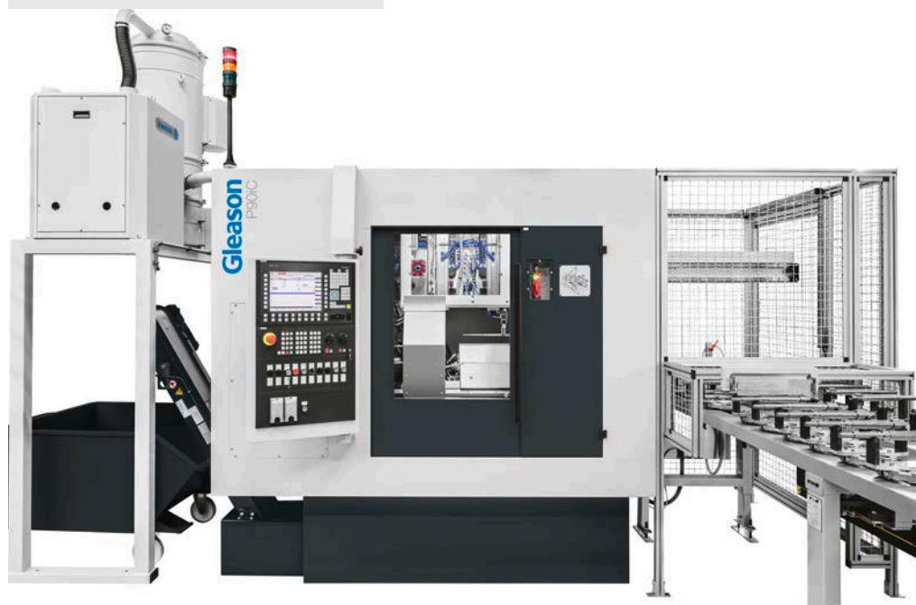
Hobbing and chamfering in one setup.
