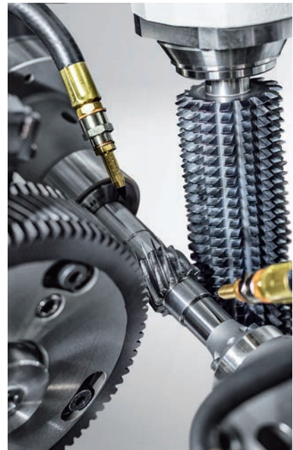
Hobbing and chamfering in one setup.
