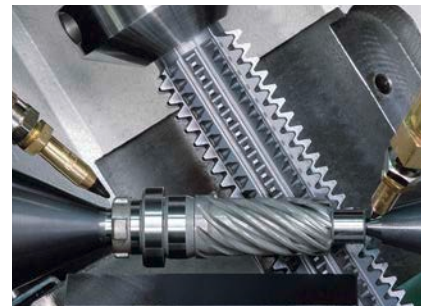
Skive hobbing of a steering pinion with a carbide tool.
