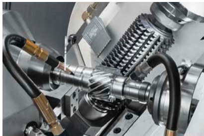
Hobbing an output shaft.
