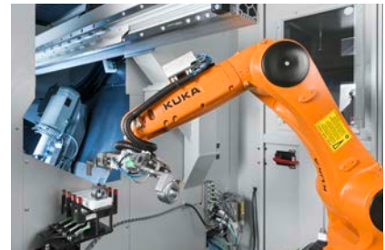
Cell integration via robotic loading.
