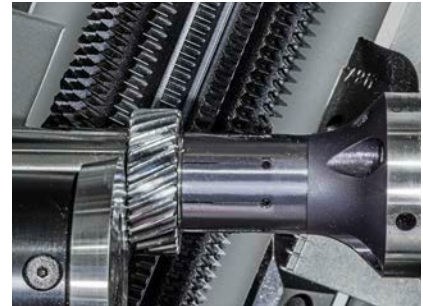
Dry hobbing and chamfering/deburring.
