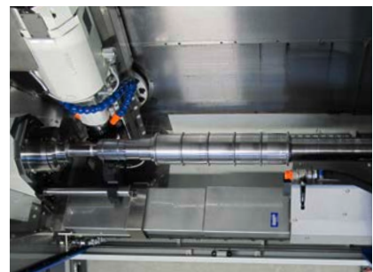
The P90EL features an extended machine frame and increased axial slide travel (cutting length) to 800 mm for shafts up to 1,200 mm in length.
