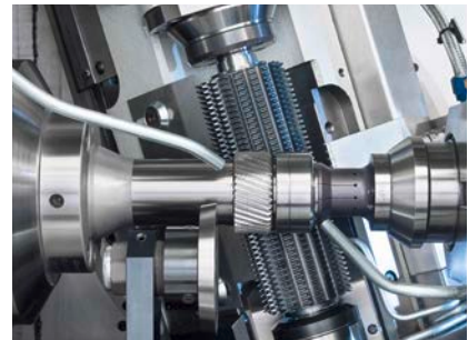
Hobbing and deburring as a dry-cut process.
