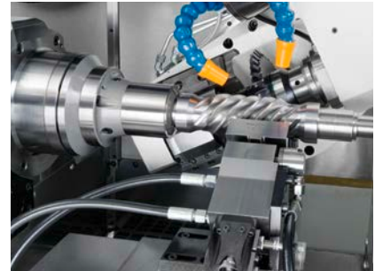
Prismatic supports are available for longer workpieces.
