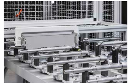
Ring-conveyor with adjustable pallets.
