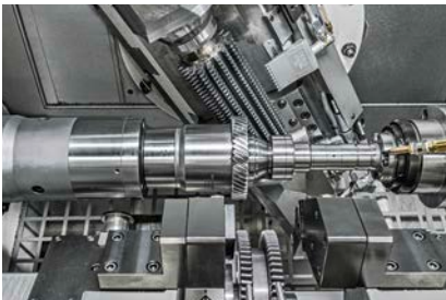
Hobbing and chamfering/deburring of an automotive input shaft.
