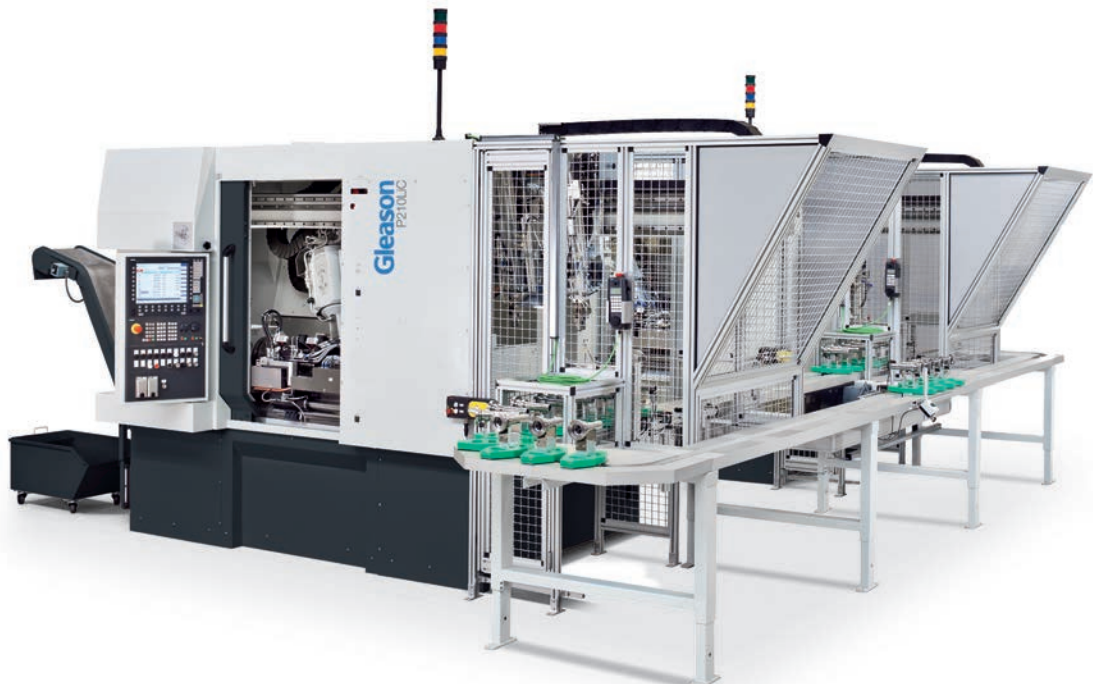
Hobbing and chamfering/deburring of an automotive input shaft.
