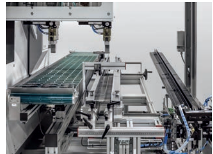
Automation with gantry, discontinuous chain belt, loading rail and unloading belt.
